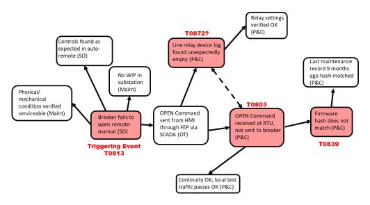
Figure 4: Example CyOTE Observables Link Diagram
